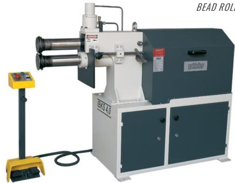
IBKS 4.0 Hydraulic bead roller model (9 gauge)
