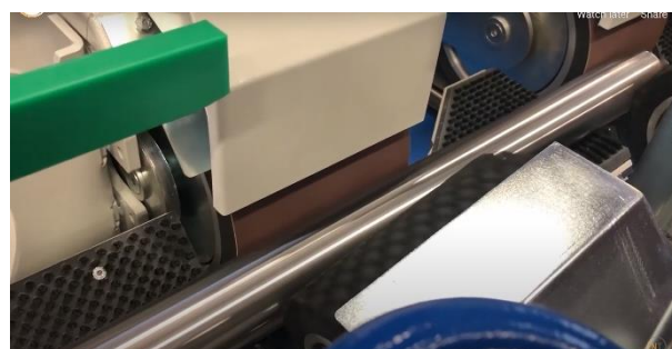
128 DL Double head pipe sander \varnothing 3/8" - \varnothing 6" Roughing and finishing in one pass thanks to dual sand belt system
