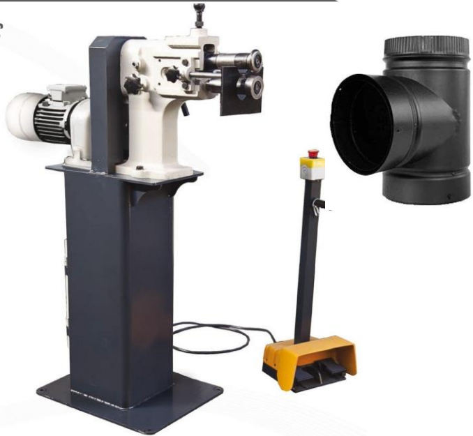
IKMP1.2 trimming and bead rolling model :18 gauge
