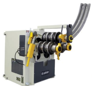
HPK 120 corrugated sheet roll bender (optional rolls)
