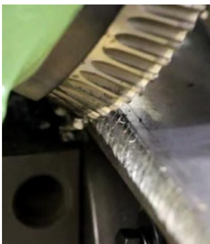
CHP 21G Max Bevel width: 1 1/8" Max Material Thickness: 2"
