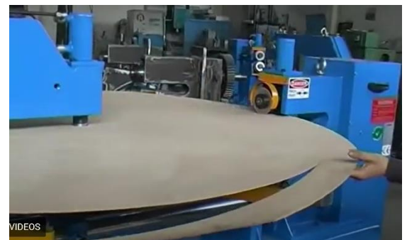
IDK 5 hydraulic Circular cutting shear (thickness: 6 gauge - Diameter: 47") motorized center adjustment and hydraulic cutting and lamping
