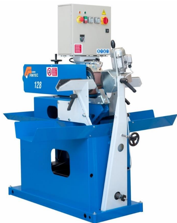
128 SL single head pipe sander \varnothing 3/16" - \varnothing 6"
