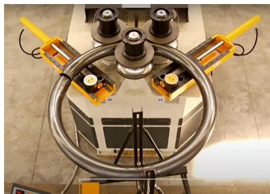
HPK DP Double pinch heavy duty roll bender (6" - 16" pipe)
