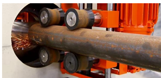
Variable speed feeder
