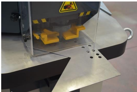
30° to 140° variable notching angle Max Punching thickness : 3/16"
