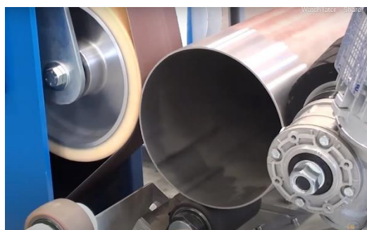
128 SL single head pipe sander \varnothing 3/16" - \varnothing 6"
