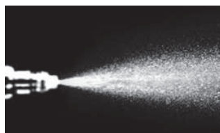
Injector spray pattern after P.i. treatment.
